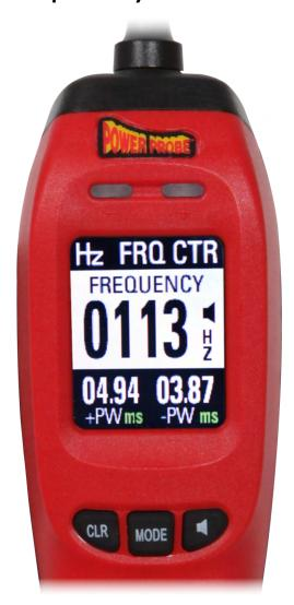
**Hz FRQ CTR** – Frequency Counter mode is used for measuring the frequency of an alternating voltage signal.
