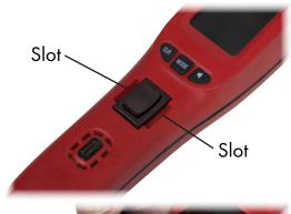
Locate the two slots on either side of the Rocker Switch.
