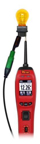
Activating Electrical Components in VDC Mode is one of the main features that make the Power Probe IV very useful when testing. Being able to apply battery power or ground right to the probe tip gives you the ability to activate and dynamically test electrical components such as lights, motors, and solenoids.
