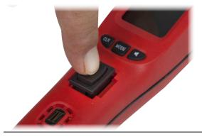
Position the new Rocker Switch into the switch cavity and carefully press straight down until the switch is flush with the housing.
