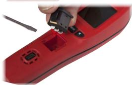
Carefully remove the Rocker Switch with an appropriate pry tool or small screwdriver. Do not apply excessive force.
