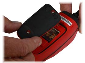
Unscrew the two retaining screws and remove the rear cover.
