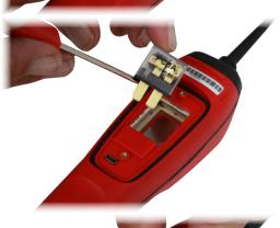
Once the Circuit Breaker is loose from the terminals, carefully lift the breaker from the housing cavity.
